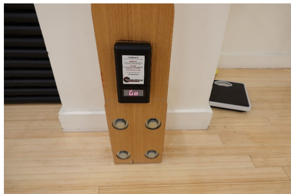
Figure 2. StrikeMeter installed at the bottom of makiwara
